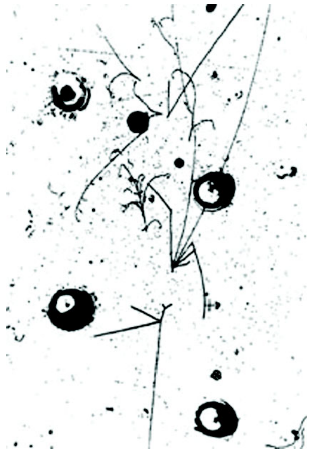
Fig. 3: A 7 GeV proton enters the Gargamelle bubble chamber from below and induces a three-step neutron cascade.
